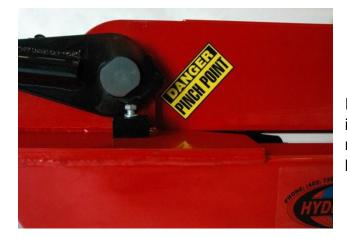
Illustrated to the left: A hazard warning indicating a potential pinch point found near the intersection of the lifting arm, handle, and frame.
