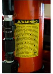
Illustrated below: A sample of the hydraulic hose warning, found on the hydraulic hose and typically most easily viewed through the Head Tilt Access Latch Door.
