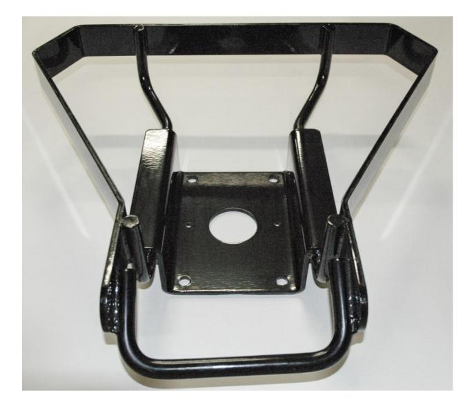
The Tri-Link adapter is a hydraulic pump removal tool for the CAT 797 Haul Truck Hydra-Tech PN # 117120012
