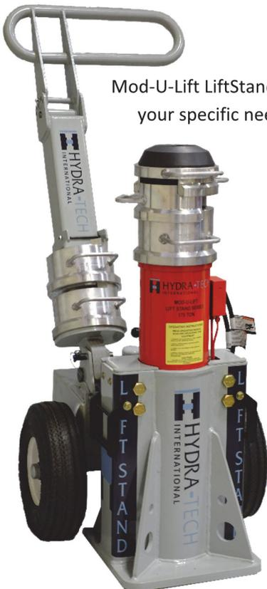
Mod-U-Lift LiftStand Series are offered in a variety of configurations to meet your specific needs. Lift Modules come in a range of 60, 100, and 175 ton capacities with various stroke lengths
