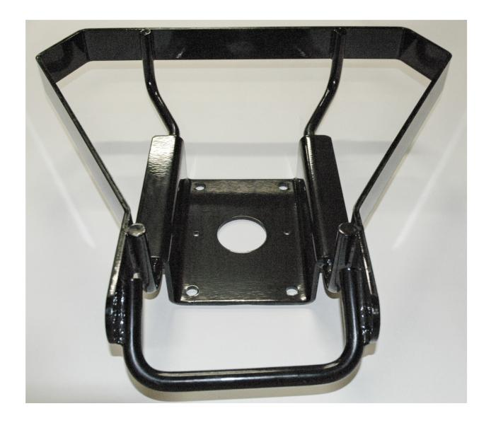
The Tri-Link adapter is a hydraulic pump removal tool for the CAT 797 Haul Truck
