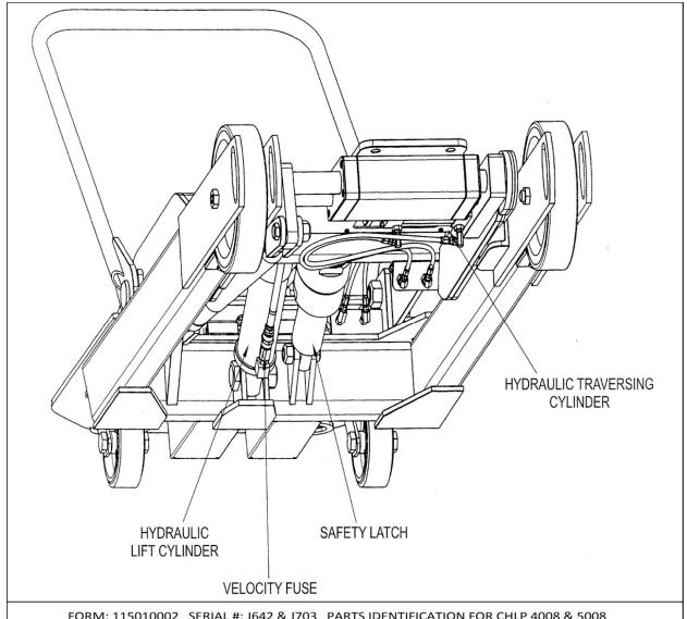
FORM: 115010002 SERIAL #: J642 & J703 PARTS IDENTIFICATION FOR CHLP 4008 & 5008 ASSEMBLY #: 115150005 & 115150007 REVISION: A DATE: 08/15/2000
