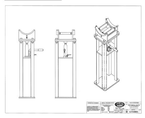
The Hydraulic Pump Adapter is used as a removal tool for CAT 797B Haul Trucks.
