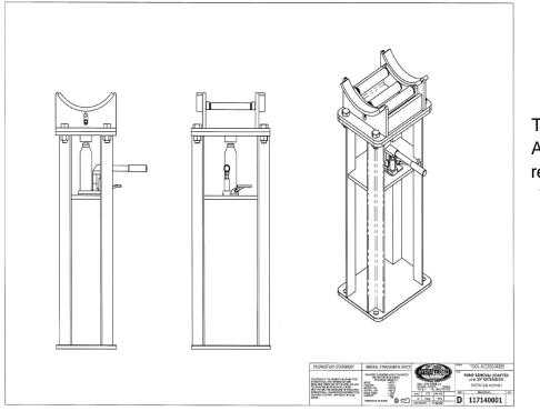
The Hydraulic Pump Adapter is used as a removal tool for CAT 797B Haul Trucks.
