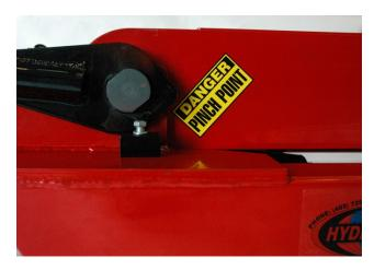
Illustrated to the left: A hazard warning indicating a potential pinch point found near the intersection of the lifting arm, handle, and frame.
